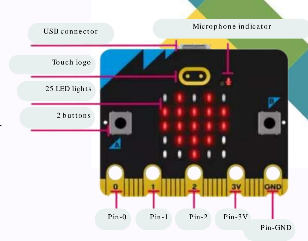
LED Display and Light Sensor - 25 LEDs arranged in a 5 x5 grid. The LEDs can be used for displaying pictures, words and numbers. They can also act as sensors and measure light levels.
