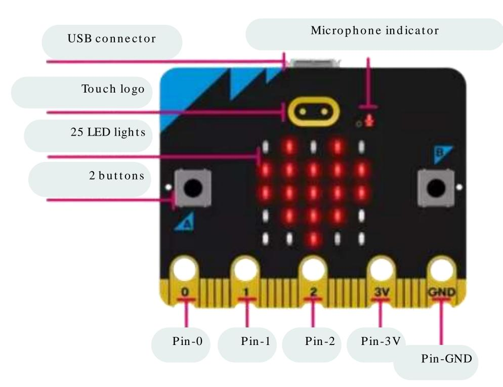
Input and Output Pins - micro:bit contains small holes on the edge. These are called pins and these pins can be split into three categories: GPIO; 3V power; and GND.
