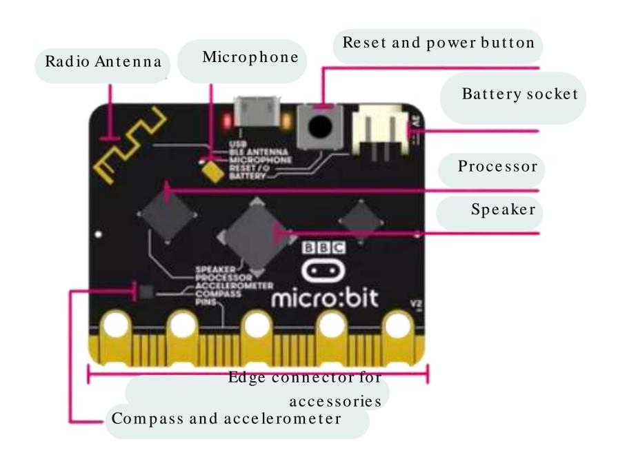
Battery - powered using a battery pack. Instead of using a computer to power it, the battery pack can be plugged into the micro:bit.
