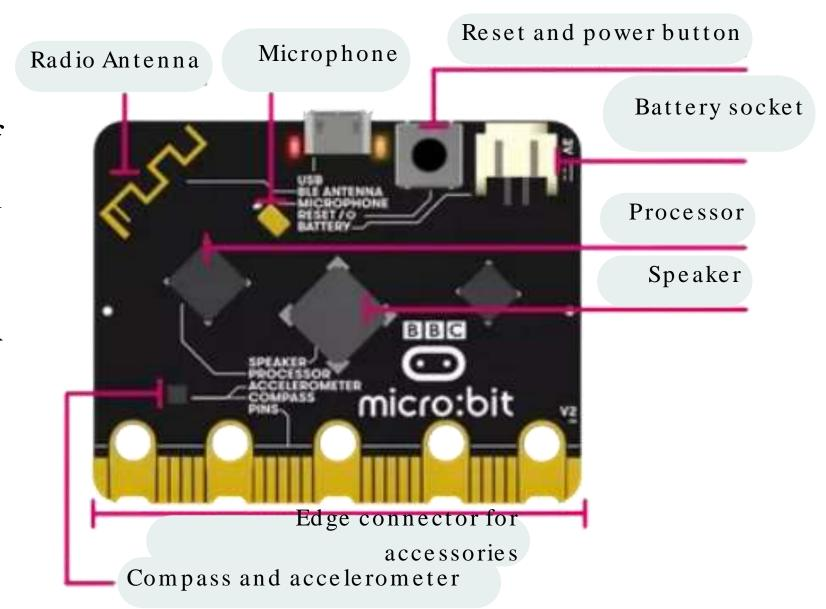
Accelerometer - contains a motion sensor that measures movement. The accelerometer can detect when the micro:bit is tilted left to right, backwards and forwards and up and down.
