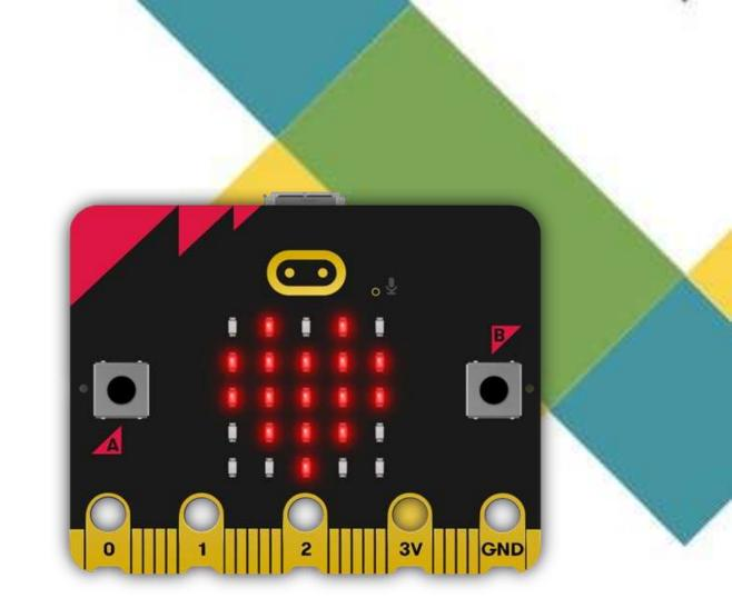
Micro USB Socket - connect the micro:bit to a computer or laptop, that allows the micro:bit to have programs transferred to it. Microphone - a has built-in microphone. The microphone LED will light up if the microphone is measuring sound levels. The microphone LED also indicates where the microphone is located.
